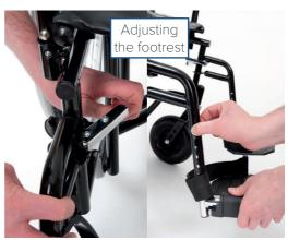
Press the brass push buttons (right) and adjust the footplates to the desired height. Release the buttons and keep adjusting the footplate until it locks in position with an audible click.
